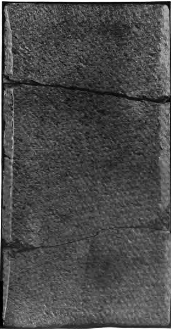
THE SHEARING STRENGTH OF STONES. Photograph of fractured specimen of Troy, N. H., granite.
